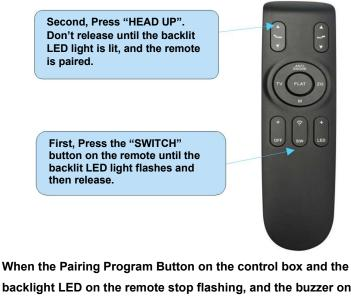
backlight LED on the remote stop flashing, and the buzzer on the control box has a "DI" sound, pairing is completed. If the pairing fails, repeat the process again.
